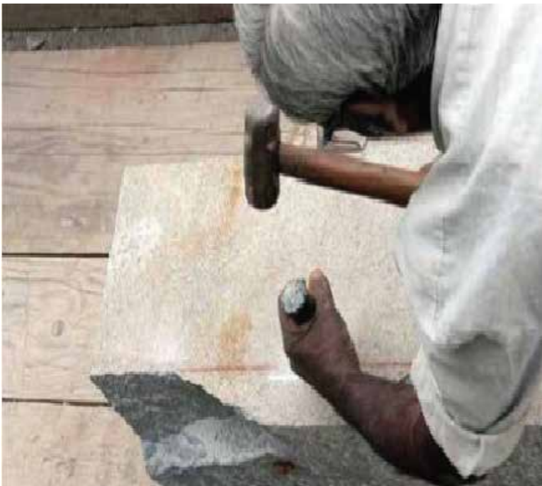
fig.21 The process of making of equipments and the different tools used in carving of stone
